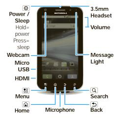
The Power key is also a fingerprint sensor. For security, you can touch Menu 📳 > Settings > Location & security > Set up screen lock > Fingerprints.
