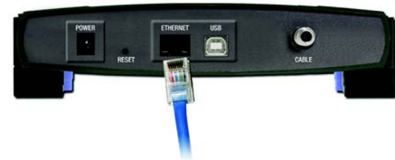
Figure 3-2: Connect the Ethernet Network Cable
