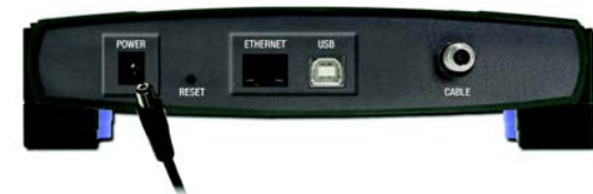
Figure 3-3: Connect the Power Cable
