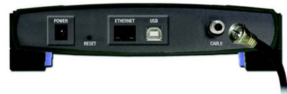
Figure 3-1: Connect the Coaxial Cable
