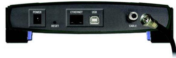
Figure 3-4: Connect the Coaxial Cable
