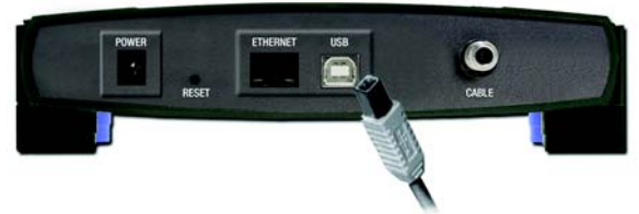
Figure 3-5: Connect the USB Cable
