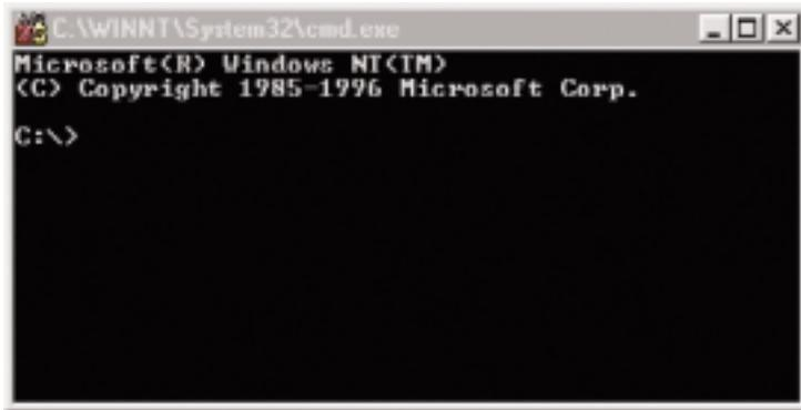
3. If your prompt does not read "C:\", type **cd..** until you are at the C:\ prompt. At that prompt, type **ipconfig /release** to release the current IP address. Then type **ipconfig /renew** to get a new IP address.
